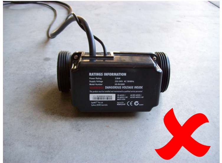
Side Install = Incorrect
