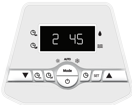
Parameter 2: Turnround if defrosting under heat mode (30-90 min). Factory setting: 45 minutes
