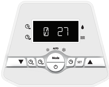
Parameter 0: Cooling setting water temperature (10-45°C). Factory setting: 27°C
